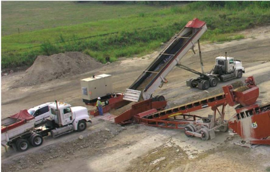
Figure 3: RazerTail® truck off-loader configuration
