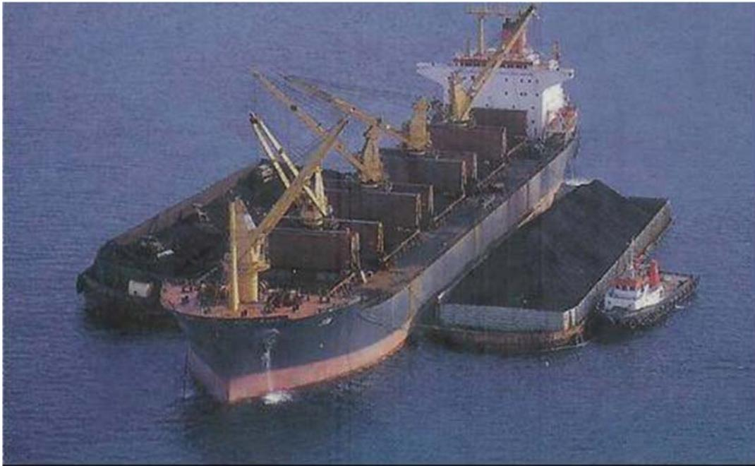
Figure 9: An example of a geared ship self-loading from deck storage barges.
