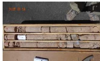
Core from 377 to 380 meters below surface showing the occurrence of a tuff layer, recently age dated by Sernageomin, within a thick sequence of clays that form the aquiclude. (13.45 ± 0.07 Ma.)
