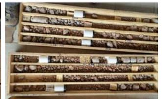
Core from 639 to 652 meters below surface showing disaggregated and missing core, from within a thick sequence of sands, conglomerates and cobbles that host the pressurized aquifer
